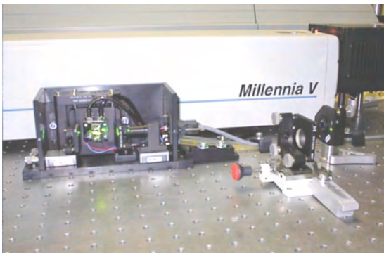
Figure 1. This X-band, 5-MeV gun (a) is the highest-frequency photoinjector currently in operation; the 10-fs laser oscillator (b) is the front end of a TW-class laser system used for producing Compton x rays.
