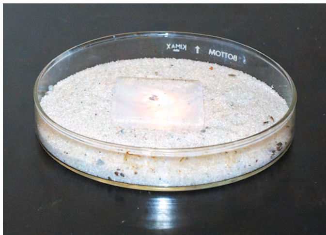
Burning iron oxide/aluminum sol-gel derived thermite atop a silica aerogel.
