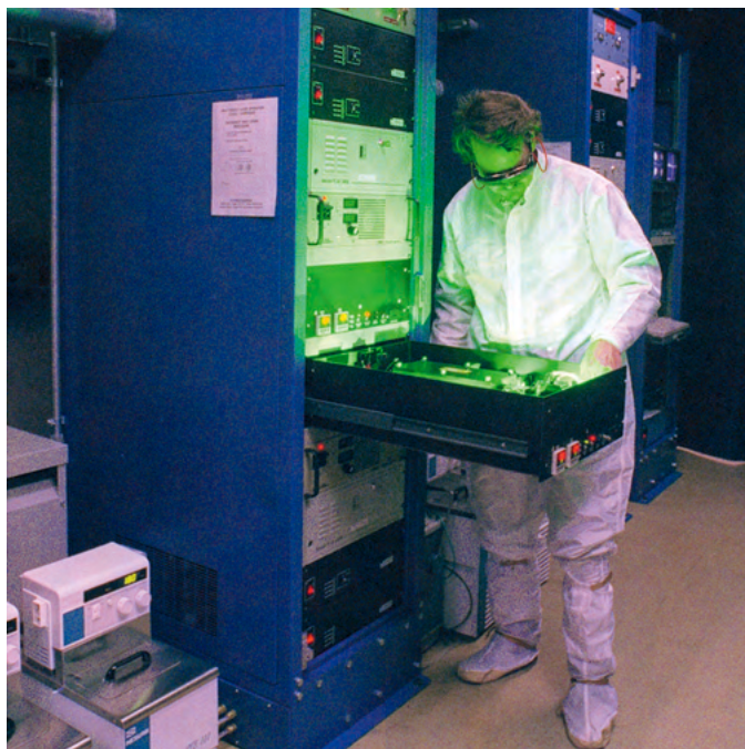
Figure 4. Diode-Pumped Solid State Green Lasers for Industrial Material Processing. Jim Chang and his team developed a cost-effective, high-powered replacement to lamp-pumped solid-state lasers.
