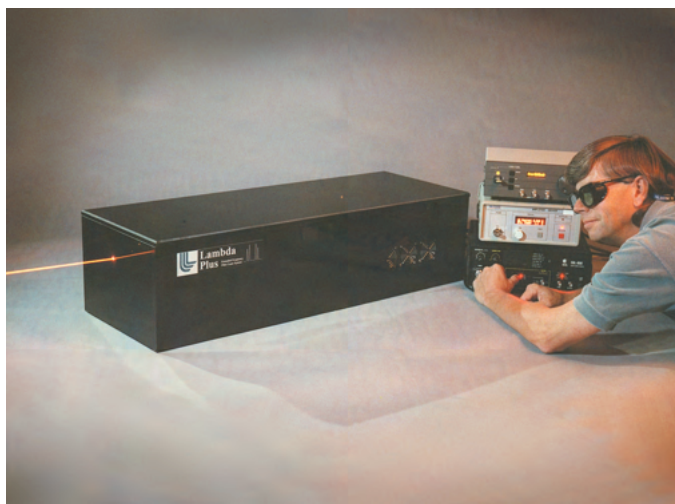
Single-frequency, tunable orange (589-nm) light beam emerging from the integrated solid-state visible light source. Electricity is the only utility required.
