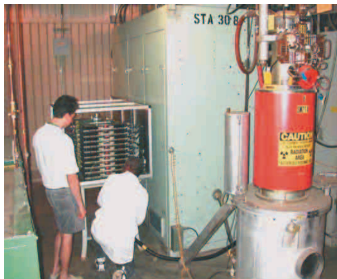
A prototype inductive solid-state modulator (left) driving a S-band klystron (right) at the Stanford Linear Accelerator Center (SLAC).
