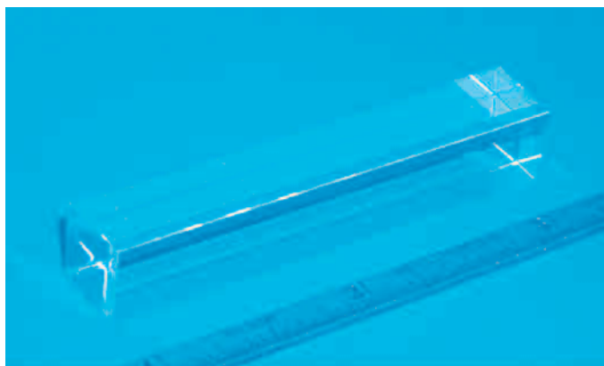
A polished section of a high-quality, small-diameter Yb:S-FAP crystal.
