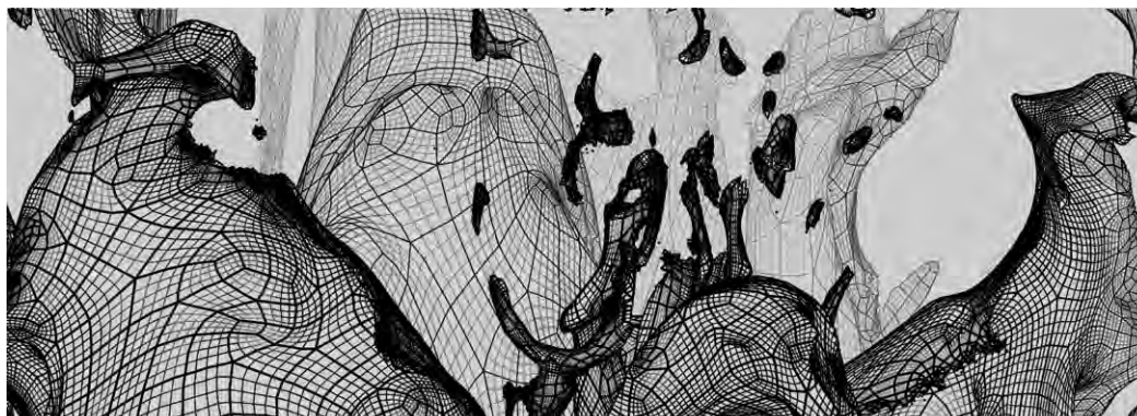
Shrink wrap of 0.3% of the mixing-layer boundary of an eight-billion-cell, turbulent-mixing simulation. Experiments show that combining shrink-wrap and wavelet compression will reduce disk storage size by a factor of 50.
