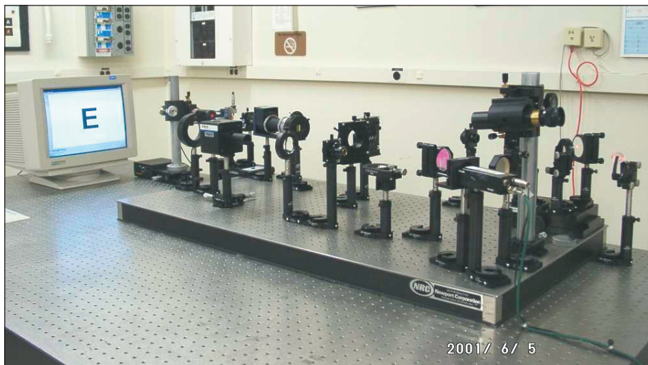
High-resolution liquid-crystal adaptive-optics system for human vision correction that will be used at the University of California, Davis beginning in FY2002 to study the limits of human visual acuity.
