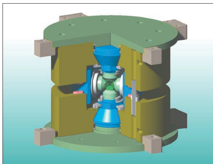
Cut-away view of the Deformation-DIA. The cubic volume defined by the tungsten carbide anvils (light green) at the center contains the sample assembly.
