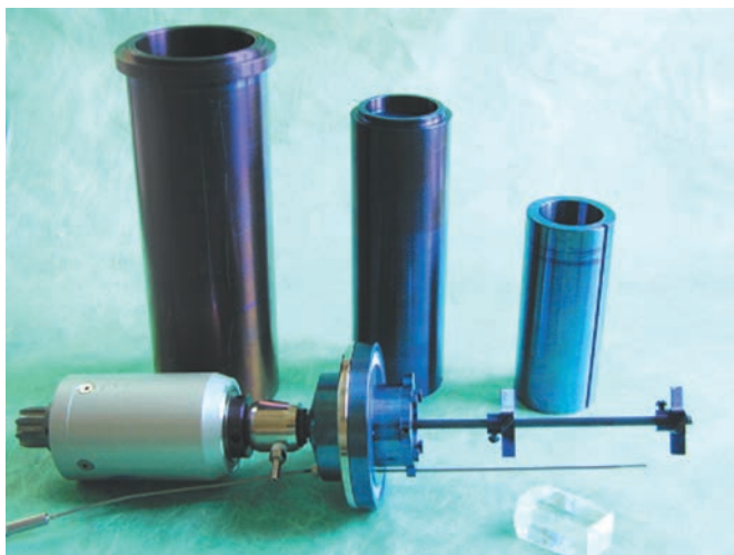
Experimental equipment being used to test the carbonate-dissolution method of \text{CO}_2 capture and sequestration, showing (a) our bench-top apparatus; and (b) a closeup of the reactor vessels (cylinders in the rear), the stirring apparatus (foreground), and calcium carbonate crystal (foreground, right side).
