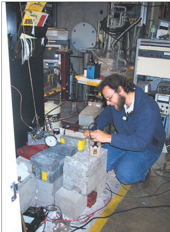
Principal investigator L. Bernstein measures prompt activity from the bromine and krypton cryotrap (dry ice and liquid nitrogen, respectively) at the Lawrence Berkeley National Laboratory 88-in. cyclotron.
