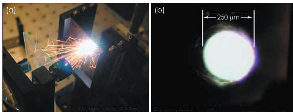
Hole-drilling experiments: (a) experimental setup and (b) photomicrograph of submillimeter hole in a 1.5-mm-thick steel substrate.
