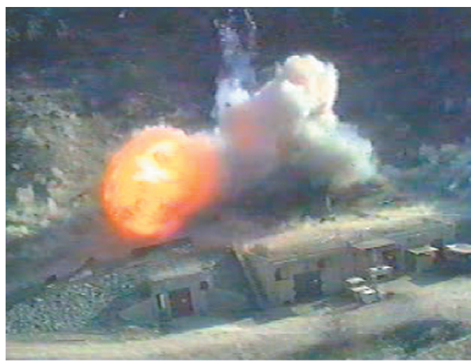
Detonation of a high-explosive, pulsed-power, isentropic compression experiment (ICE) at Los Alamos National Laboratory. The detonation of tens of kilograms of explosive generates an electrical current of several million amperes. The intense magnetic field associated with that current smoothly compresses a centimeter-size metal target to a pressure of hundreds of thousands of atmospheres.
