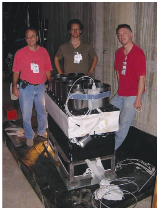
Louisiana State University collaborator William Coleman, LLNL principal investigator Adam Bernstein, and LLNL co-investigator Steve Dazeley (left to right) with a prototype gadolinium-doped water Cerenkov antineutrino detector developed to explore rare events in next-generation particle astrophysics. The device detected antineutrinos emitted from the San Onofre Nuclear Generating Station. Antineutrinos interacting in the water generate a unique pattern of faint blue flashes of Cerenkov light, which the detector records.
