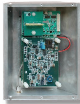
SecureBox is a wireless device that can be installed within the metal corrugation of a cargo container to detect intrusions.
