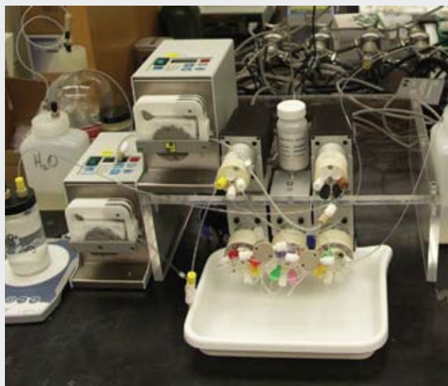
Prototype automated radiochemistry system developed for heavy-element chemistry.
