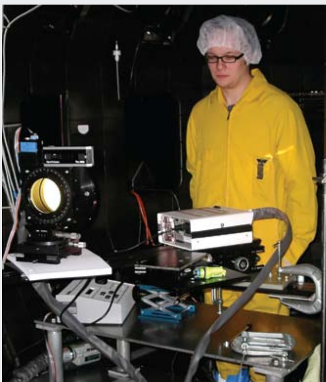
Graduate student Josh King working inside the General Atomics DIII-D tokamak fusion reactor in San Diego on the calibration of the motional Stark effect diagnostic.
