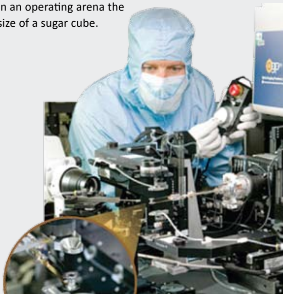
Systems engineer and LDRD investigator Richard Montesanti operates the precision robotic assembly machine. The inset shows an assembled fusion ignition target.
