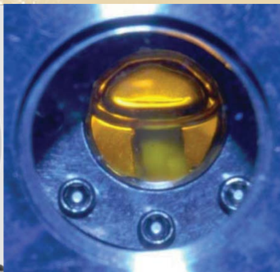
An x-ray radiograph of a 2-mm diameter, 30- \mu\text{m} -thick diamond shell with an approximately 50- \mu\text{m} layer of dicyclopentadiene polymer gel is shown (left), and a 30-mg/cm 3 dicyclopentadiene polymer foam that survived wetting with cryogenic hydrogen (right).
