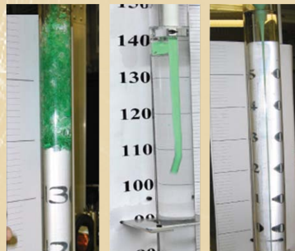
Stabilization of the turbulent breakup of descending water in oil (left) by cornstarch (middle), along with the descent of the same suspension at a slower speed (right).
