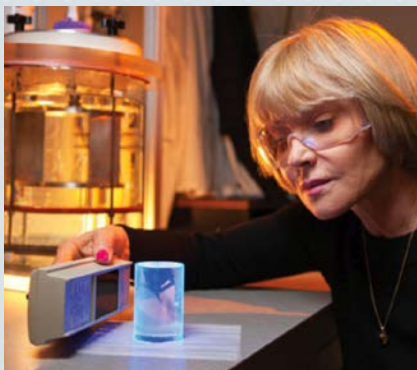
Livermore physicist Natalia Zaitseva leads a research team that has developed the first plastic material capable of efficiently distinguishing neutrons from gamma rays.
