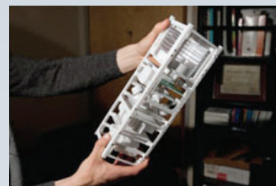
Miniature Pathfinder satellite with imaging payload.
